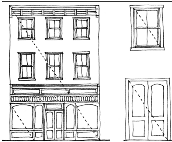
Illustration for Proportion. Analysis of three-story commercial building façade showing the repeated proportions in façade elements, beginning with the overall façade and carried down to the proportions of individual glass panes. (Geometrically, when the diagonals of rectangles are parallel, the rectangles are proportional.)
